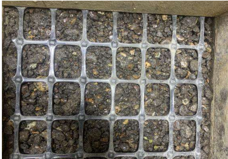
Figure 1. Biaxial geogrid reinforcement used in the study.
