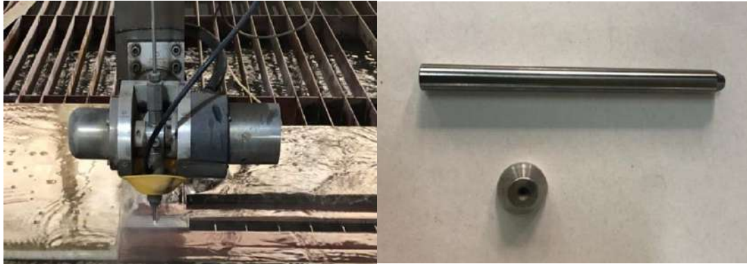
Figure 8. Depicts the cutting head and tube
